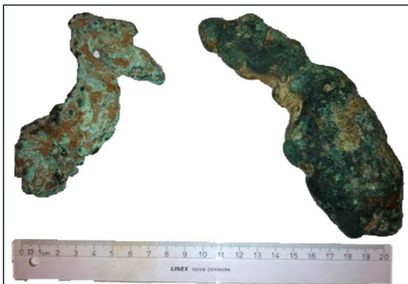
Figure 21: Large native copper specimens from ARC. Sample on the right weighs ~1 kg
